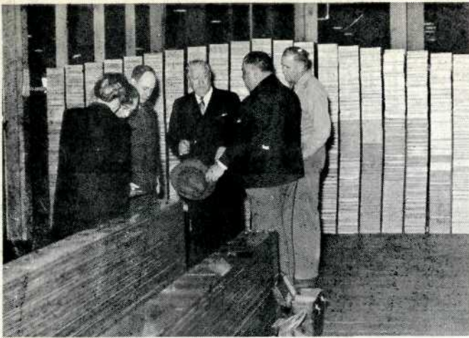
SILVER SUBSTITUTE —Early in December, 1942, approximately 141 tons of solid silver (shown stacked in slabs in picture above) arrived at BMI, protected by a unit of Federal guards. Originally mined in Nevada, the silver was substituted for copper in the massive installation of busbar, carrying electrical current of extremely high voltage necessary in the manufacture of magnesium. Senator Pat McCarran (center in the group above) visited BMI several times during construction and initiated the legislative program that kept the plant facilities in Nevada after the war ended.
