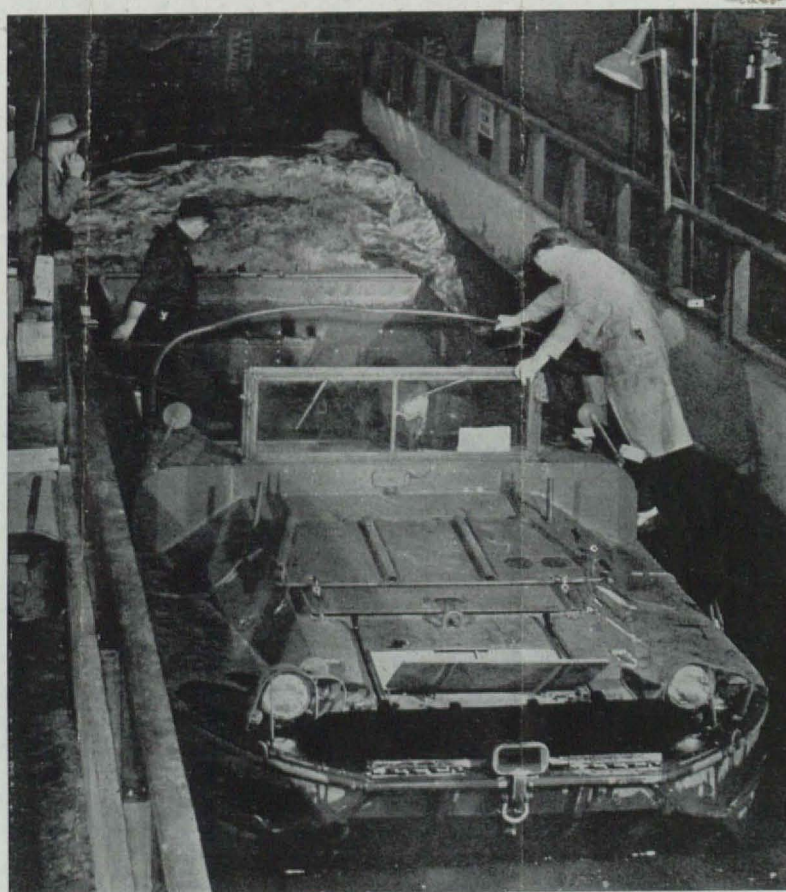
"DUCK" UNDERGOES TEST: Amphibian trucks can pull themselves out of mud or quicksand with astonishing ease by means of a power-driven winch. Winch cable is attached to a tree, post or any solid object and the engine-driven winch does the rest. Above, the amphibian is being subjected to the "bathtub" test for water leaks at General Motors Truck and Coach factory
