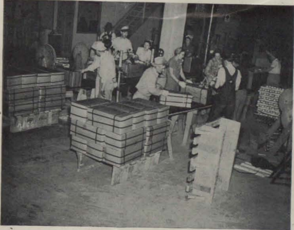
In shipping department, finished ingots are strapped with steel and packed into cardboard cartons for shipping.
