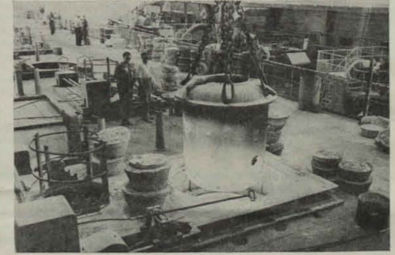
(Above)—Various alloys are made at the BMI refineries—for incendiary bombs, sheet magnesium, airplane parts, tracer bullets, and flares. This crucible, freighted with two tons of white-hot magnesium alloy, has just been lifted from the gas furnace and is being lowered into a cooler before being transported to the ingot pouring machine. (Below)—F. O. Case, general manager of BMI, presents an incendiary bomb made of Basic metal to Major Robert Morgan, pilot of the famed Memphis Belle, the flying fortress which made 25 trips over Germany. Major Morgan told BMI workers: "O. K. You made it and we'll deliver it."
