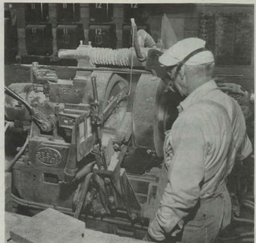
Easley grinders cut brick into 260 different shapes required for plant construction.
