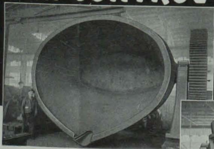
● 175-Ton Hot Metal Holding Ladle built by Treadwell Construction Co., Midland, Pa.
