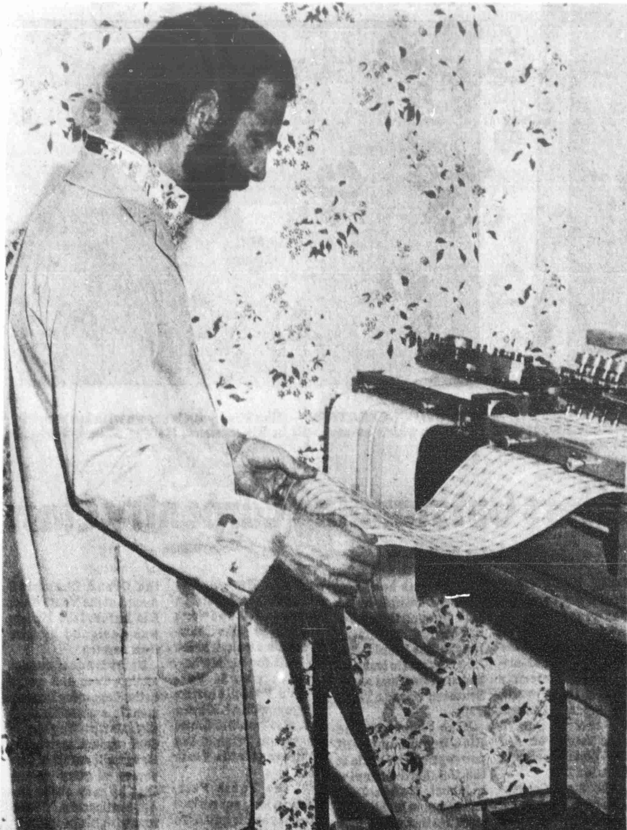
MOMENT OF TRUTH - Fisher Pen's Chuck Woodworth inspects the test writings of a group of newly manufactured points at the Fisher Pen Company operation in Boulder
