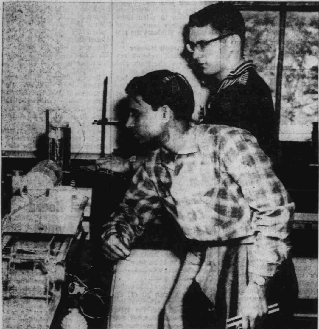
PARTNER FROM INDIA — Here Jerry is preparing single crystals of tin for a laboratory experiment on crystal growth. His partner in this experiment is G. P. Ramulu of Hyderabad, India, a senior student in metallurgical engineering.
