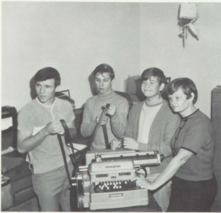
Joe Babcock, Mike Fuller, Bob Anderson, and Mrs. Anderson, examine tape from Flexiwriter before they feed it into the computer
